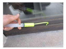
Apply the with water diluted fluorescent dye between fine gaps, in cracks or window frames with the help of the included dosing hose.
