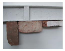
"Reaxyl<sup>®</sup> ZX-345 can also be used for gluing full bricks, without any support, in every direction and on diverse surfaces."
